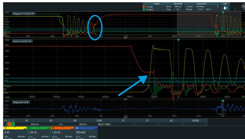
(b) Magnification of the glitch on the B trigger
