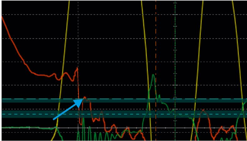
As shown in the figure, there is quite a bit of dead time, a quality often seen in bidirectional charger test setups. The resonance during the dead time shows glitches on both gate signals, resulting in a failure of the trigger to capture the time interval of concern. Raising the trigger level for channel 3 will not work in this instance because it violates the correlation in timing between channels 2 and 3.
