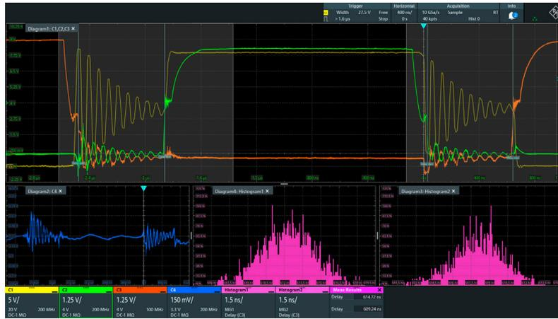
In order to trigger on a specific dead time, an A-B-R trigger (normal mode) can be set up (Figure 13) as follows:
